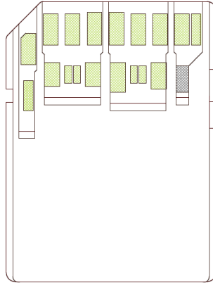
Figure L-3 : Standard SD Express G4L1 (Gen 4 1 lane) Card simplified view of pads side
